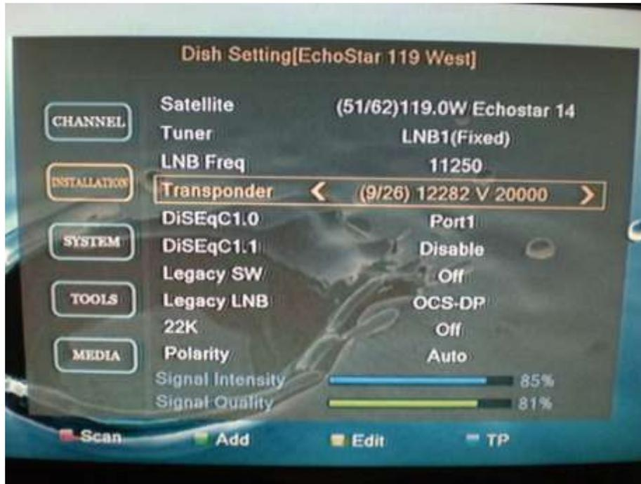
My setup shows how to set up D Pro Plus antenna such as 1000.2 WA
