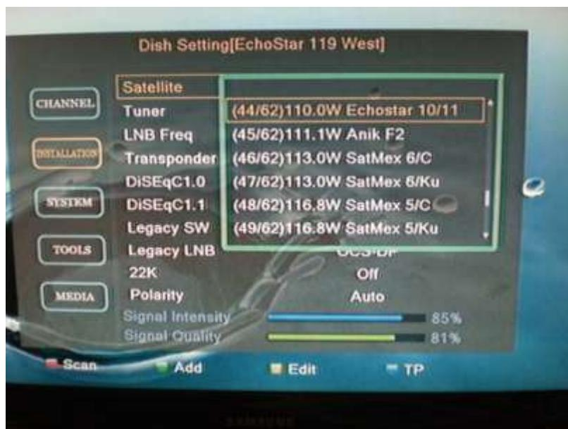
The top satellite will not be the one you want. Press (OK) and another box will open up with all the satellites in it. Use the up and down arrow to select the satellite you are configuring, and then hit OK.
