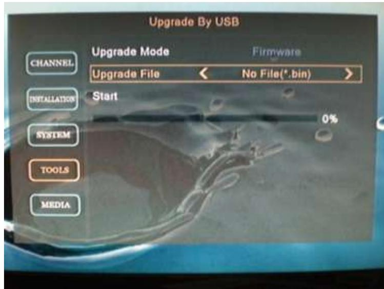
Left and right arrow keys can change the Upgrade mode. It needs to be on **Firmware** for this operation.
